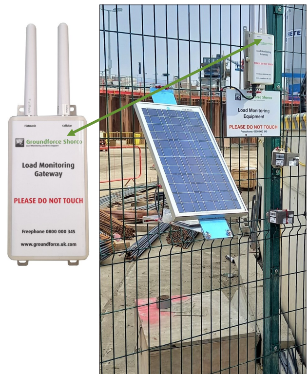
The 3G Gateway initiates the connection with the FlatMesh™ WebMonitor™ software so that the data can be viewed remotely via the internet using the FlatMesh™ WebMonitor™ Portal.
