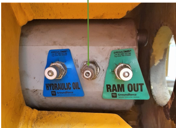
View of the hydraulic couplings through the strut housing
