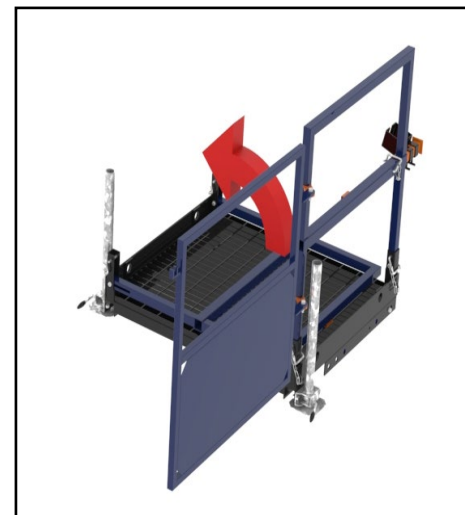
STEP 3: REMOVE RAPID PINS FROM BASE, STAND UP INTO POSITION. FRAME DROPS INTO BASE, REPLACE RAPID-PIN TO SECURE.
